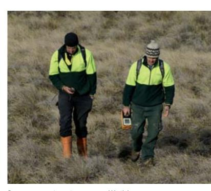
Gamma ray spectrometer survey on L'Antioja
