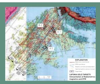
Lafonia Project - structural interpretation (Radiometric, Magnetic and DTM)
