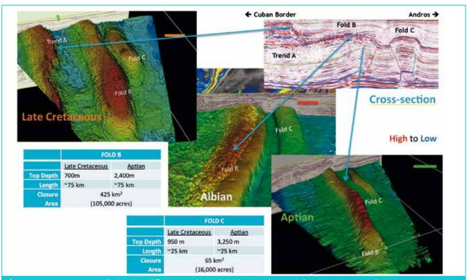
Figure 1 3D structure maps displayed at different stratigraphic horizons and related directly to the 3D section.
