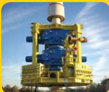
HWCG – 18 3/4” 15K dual ram “Capping Stack” unveiled by oil industry partners led by Exxon.
